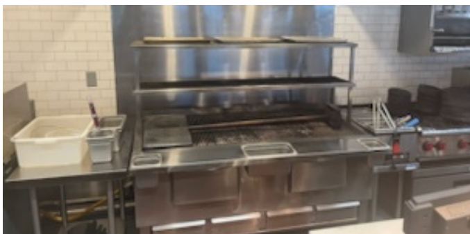
Double SS Overshelf with Cast Iron Grill Grates for the shelf units. 34-72"
